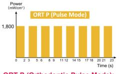
**ORT P (Orthodontic Pulse Mode):** 1,800 mW/cm<sup>2</sup> ( $\pm$ 10%) of light turns on for 2 seconds and then off for 1 second eight times
